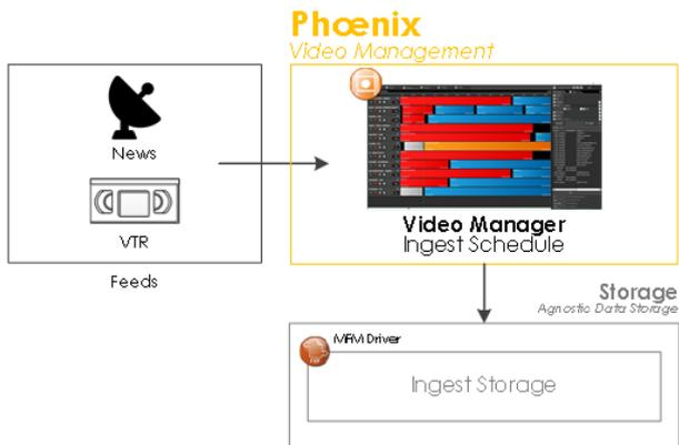
The Phoenix Video Manager offers the possibility to manage live programs through Crash or Scheduled Recording. Tape ingest is possible by controlling VTR's or a robotic solution.
